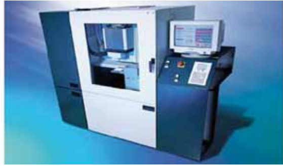
Fig. 15b. Lava™ form Computer-aided milling machine.
